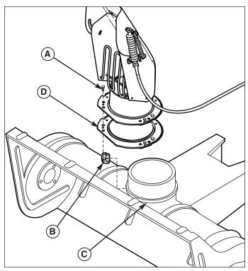
Figure 11. Assemble Discharge Chute
